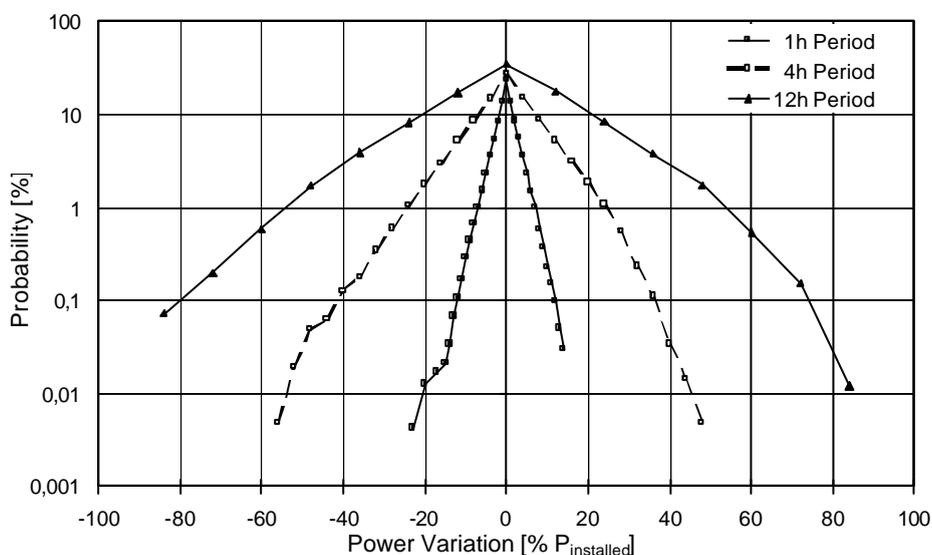
**Fig. 11: Probability of Mean Power Changes (1496 WTs) [3]**
