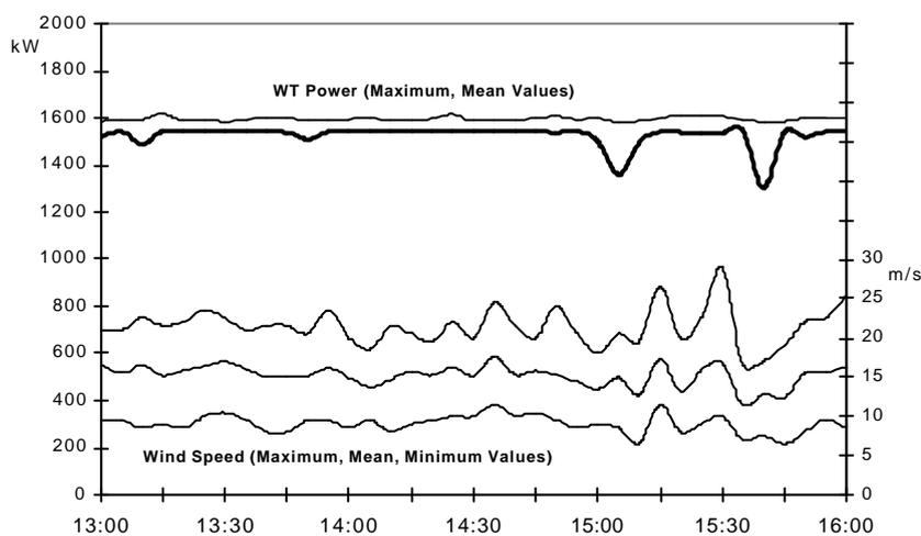
**Fig. 8: Short-term Maximum Power from WT (1.5 MW Rated Power), Variable Speed Operation [3]**
