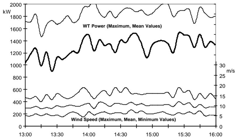
**Fig 7: Short-term Maximum Power from WT (1.5 MW Rated Power), Constant Speed Operation [3]**
