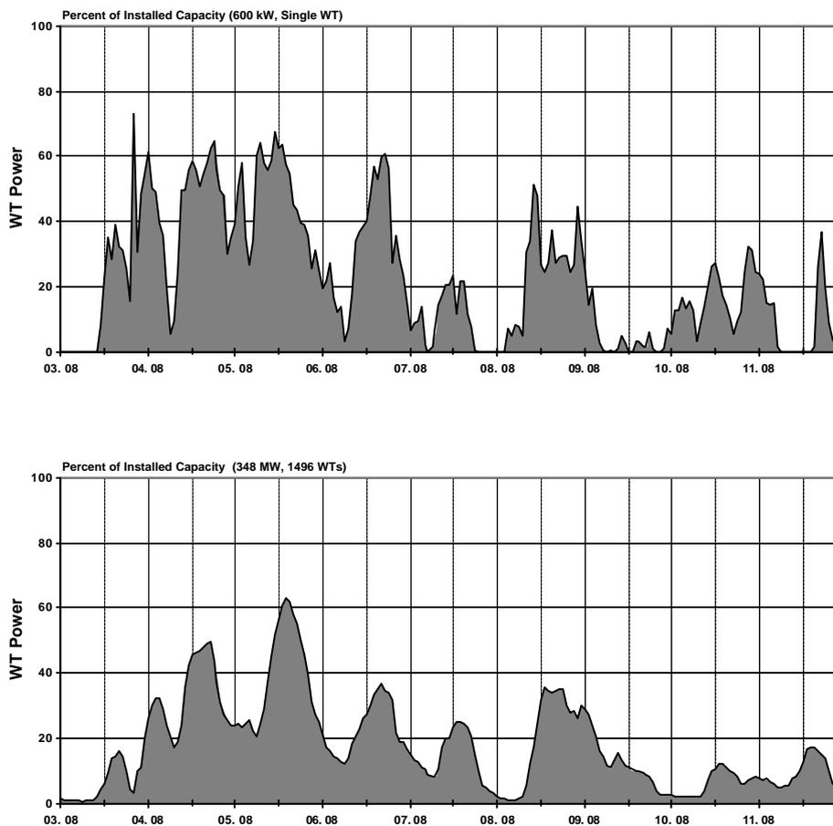
Fig. 9: Comparison of WT Individual and Cumulative Power [3]
